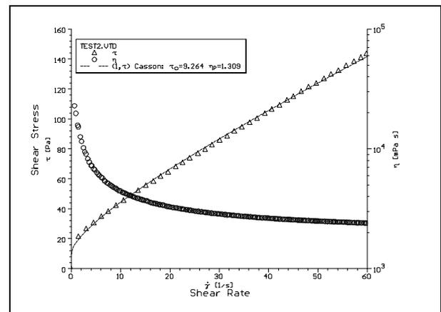
Fig. 1: Typical Flow and Viscosity Curves of a Milk Chocolate Coating at 40°C
