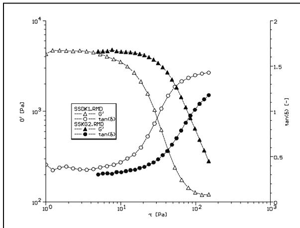
Fig. 3: Oscillation Stress Sweep on 2 different toothpastes
