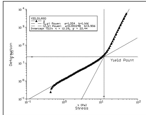
Fig. 2: Yield Point determination from a stress ramp
