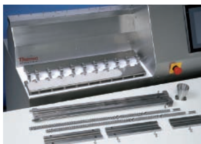
Removable contact parts for quick product changes.
