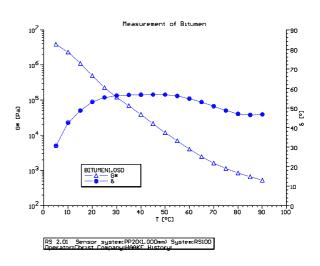
Fig.2: Temperature behavior of Bitumen
