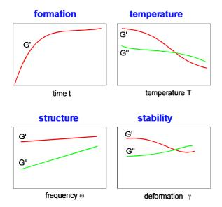
Fig.1: Schema of the storage moduli G' and the loss moduli G" as function of various measurement parameters as well as the possibility of correlation with sol-gel characteristics.
