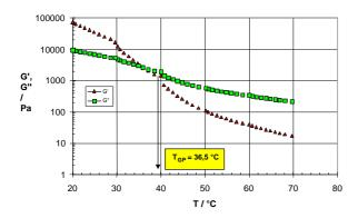
Fig. 2: Storage modulus G' and loss modulus G' as a function of temperature T for the tested gelatin (angular velocity  $\mathbf{w} = 2,15$  Hz, cooling rate 5 K/min); every 10 degrees MultiWave-measurement (0,215-10 Hz).
