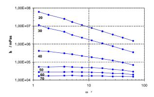
Fig. 5: Dynamic complex viscosities  $\mathbf{h}^*$  as a function of angular velocity  $\mathbf{w}$  at different temperatures T for the tested gelatin (measuring results from MultiWave-measurement (0,215 - 10 Hz).
