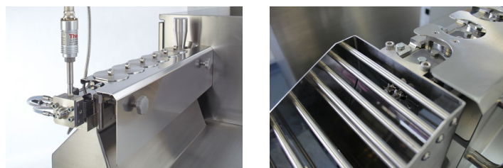
Thermo Scientific Pharma 16 Twin-Screw Extruder set-up for HME (left) and TSG (right) operation
